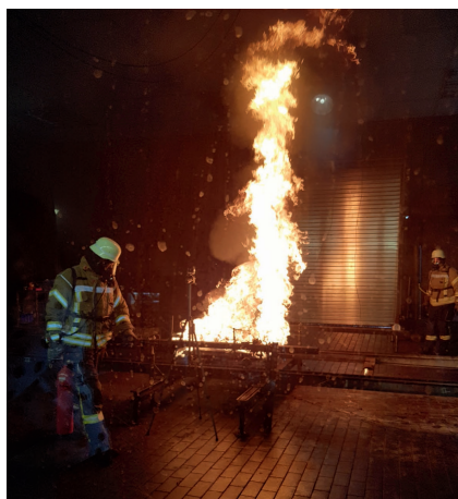
Fig. 4. The material must withstand temperatures of up to 800 °C in the fire test. This ensures that the battery does not catch fire
